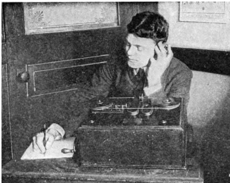
Operator and clockwork (note crank handle, lower left) magnetic detector Credit: Wikipedia
